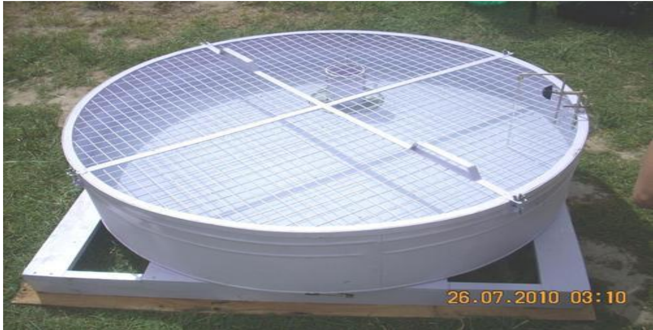
Figure 1: (I.S. 5973-1970) EVAPORATION PAN WITH FIXED POINT GAUGE AND MEASURING CYLINDER
